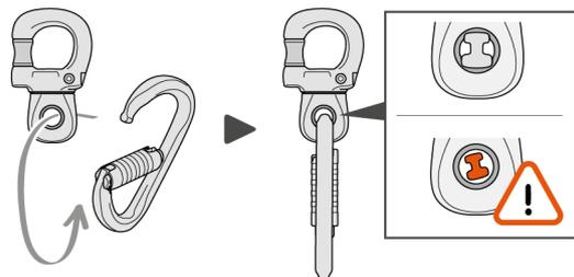
**7. Installing the swivel connector
