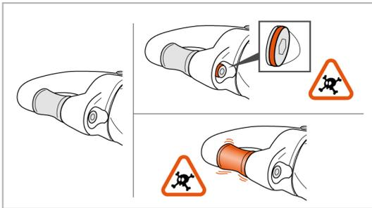
Installing the connector
