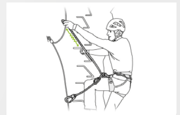
Long extension capacity and elastic arms for easier progression and to adapt to different user heights.
