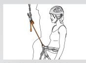
Adjustable and compact single lanyard for tethering to the anchor when climbing and mountaineering.
